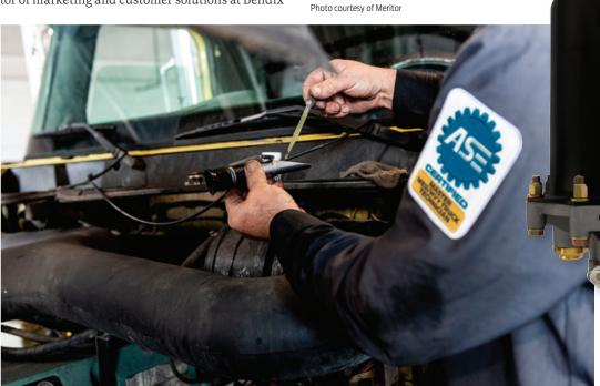
» Some engines can lose gallons of glycol in a year, so freeze levels must be checked during a vehicle's scheduled PM, especially before winter.
