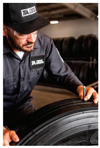
» Fleets should use a tread depth gauge to check each tire, and replace tires that are on the borderline or beyond. The U.S. DOT specifies minimum legal tread depths of 4/32" for steer tires and 2/32" for all others.
