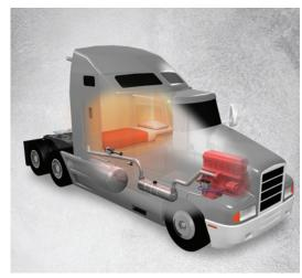
» Using an air heater instead of idling the vehicle's engine can save fleets on fuel costs and reduce engine wear and tear.
