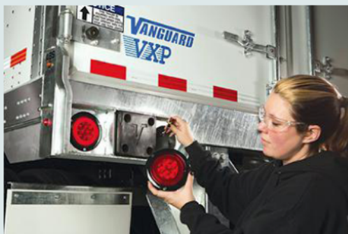
Regularly check trailer light wiring and insulation for cracks.
