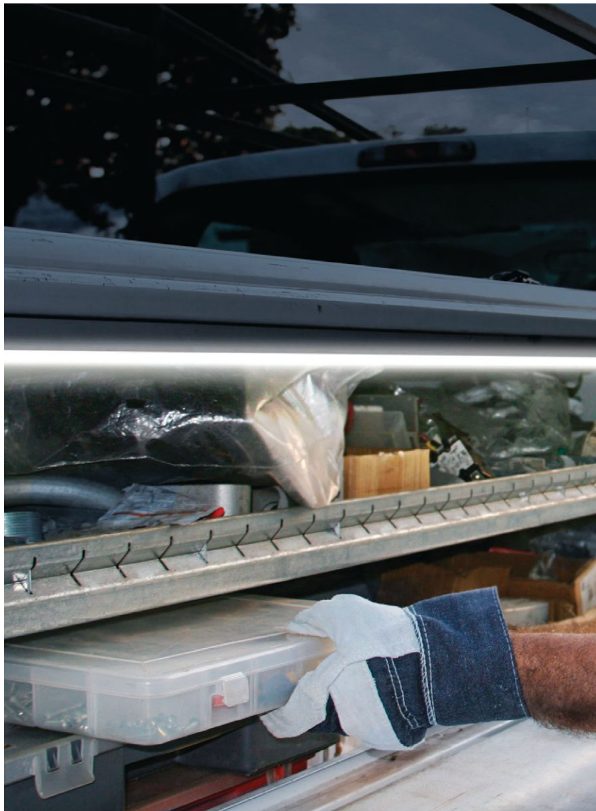
▲ Optronics' Heavy-Duty LED Silicone Rope Light lets workers avoid potential injuries from tools and sharp objects lurking in otherwise dark and unlit compartments.
